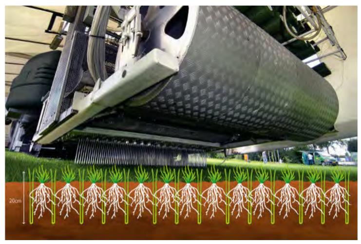
PLASTIC FIBERS INTERWOVEN INTO THE NATURAL GRASS ROOT MATERIAL TO PROVIDE SUPPORT AND STRENTGH
